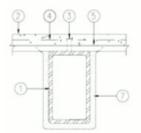
1. **Steel Tube Beam** — ASTM A500 tube beams (46 or 50 ksi) having an A/P between 0.267 and 0.616. The minimum tube dimension shall be 4 in. and the maximum tube dimension shall be 12 in. Both square and rectangular sections permitted. When rectangular sections are used, tubes shall be installed vertically with one narrow face secured to the steel floor and form units (Item 5).
