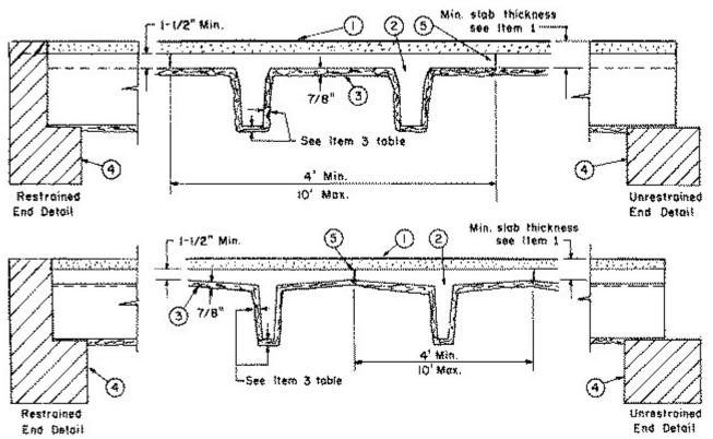
1. Concrete Topping — (Optional) — 3000 psi compressive strength, 110 to 153 pcf unit weight. Minimum topping thickness — 1 in.
