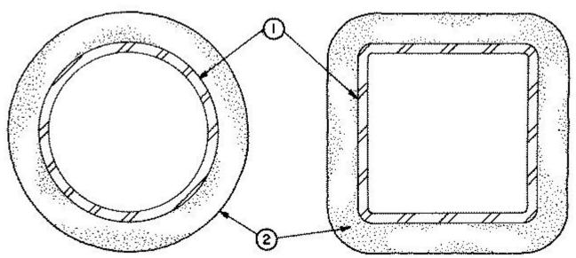
1. **Steel Pipe or Tube Column** — Steel circular pipe (SP) with diameter (ID) ranging from a minimum of 3 in. to a maximum of 32 in. with a minimum wall thickness of 3/16 in.
